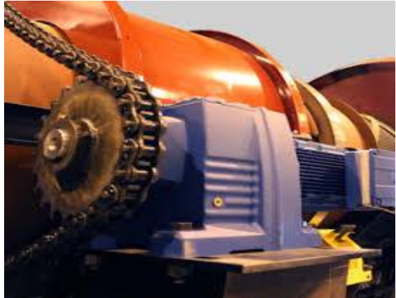
Sprocket with 52 teeth /22% reduction
